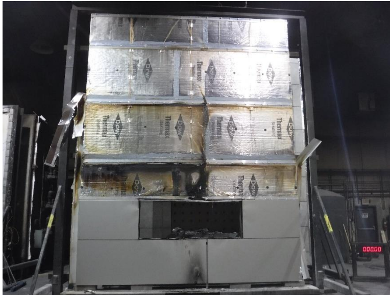
Photo No. 17 Exterior Cladding Removed
