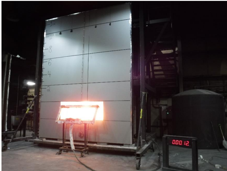
Photo No. 10 Ignition of Room Burner
